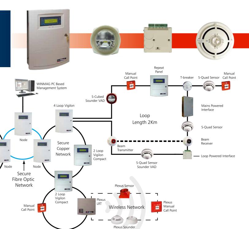
A multi-domain Vigilon Network has the capacity to support up to 200 panels per system
